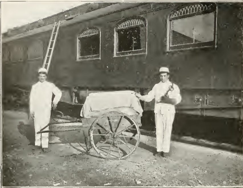
Men engaged in the work of icing cars wear white duck uniforms and gloves. The ice carts are sterilized with live steam frequently and the ice is kept covered with clean white canvas.
